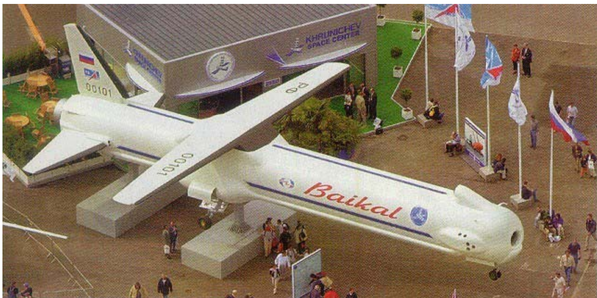
Fig. 5. The full-scale engineering mock-up of the 'Baikal' reusable fly-back booster at Le-Bourget in 2001 (Khrunichev photo).
