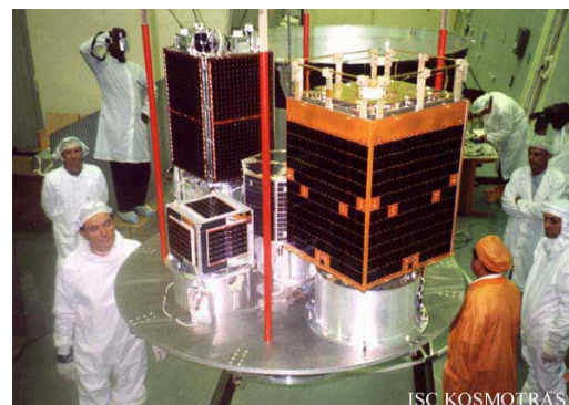
Figure 5. Platform with 5 spacecraft (Dnepr launch # 2)
