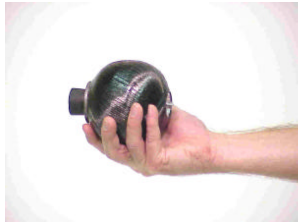
Figure 5. Nanosatellite Solid Rocket Motor Inert Model.
