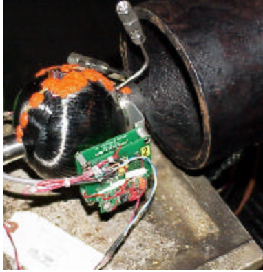
Figure 4. Pretest Setup of S/N 002 NSMP Motor Fired at Vacuum
