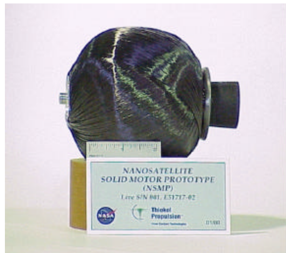
Figure 3. S/N 001 NSMP Motor Fired at Sea Level
