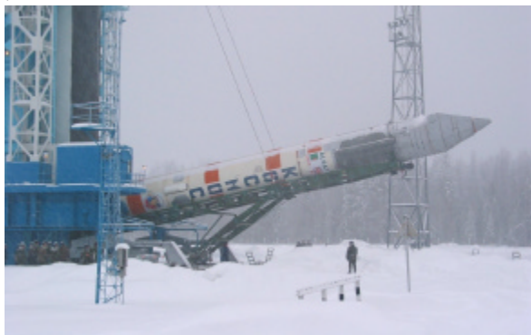
Figure 16 Kosmos launcher with ALSat being raised for launch
