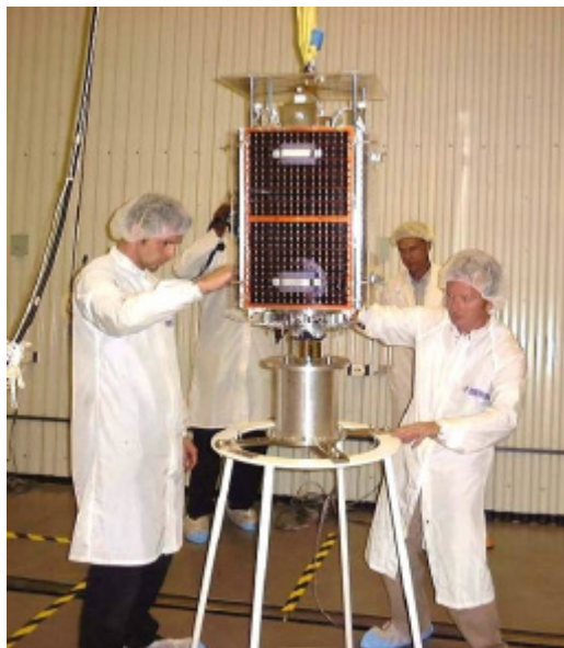
Figure 10 TiungSat spacecraft being mounted onto its interface
