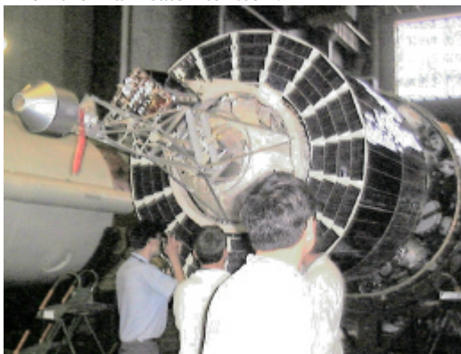
Figure 6 Tsinghua microsatellite mounted on Nadezhda main payload
