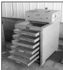
Figure 3.12 Sieve shaker for the preparation of dry aggregate
