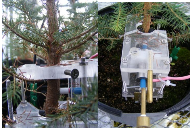
Figure 5.1 Dendrometer (showed from different angles) installed on the surface of the bark of a black spruce sapling during the greenhouse experiments in 2011 and 2012.
