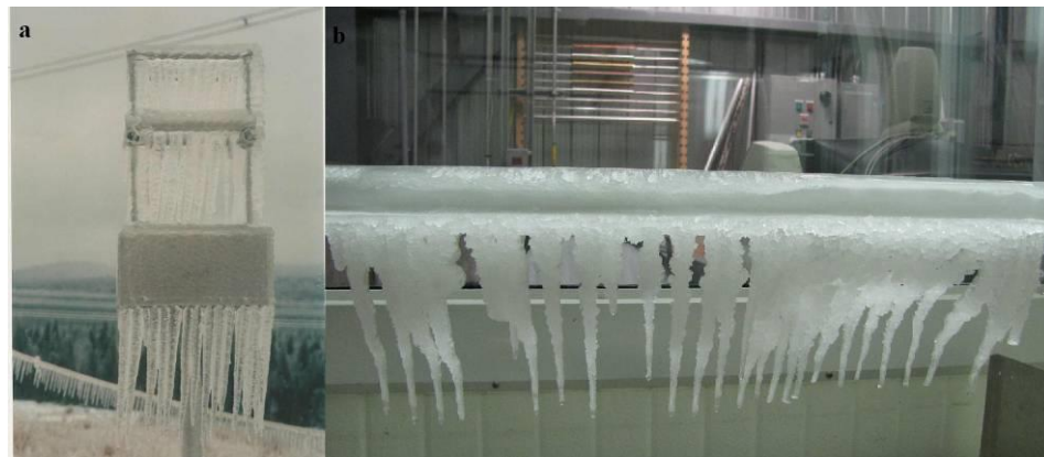
Figure 4-1: Glaze ice with icicles, a) Petite-Rivière Saint-François, b) Wind tunnel ice simulation on angle member
