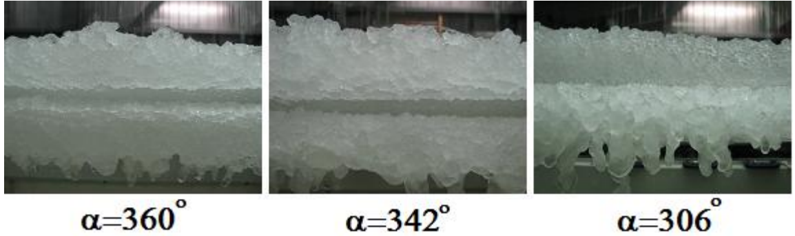
Figure 4-13: A51xL9-2 ice structure for \alpha=360^\circ , \alpha=342^\circ and \alpha=306^\circ
