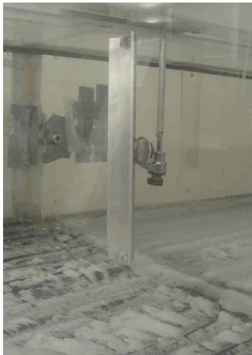
Figure 3-6: Support used for vertical ice simulation
