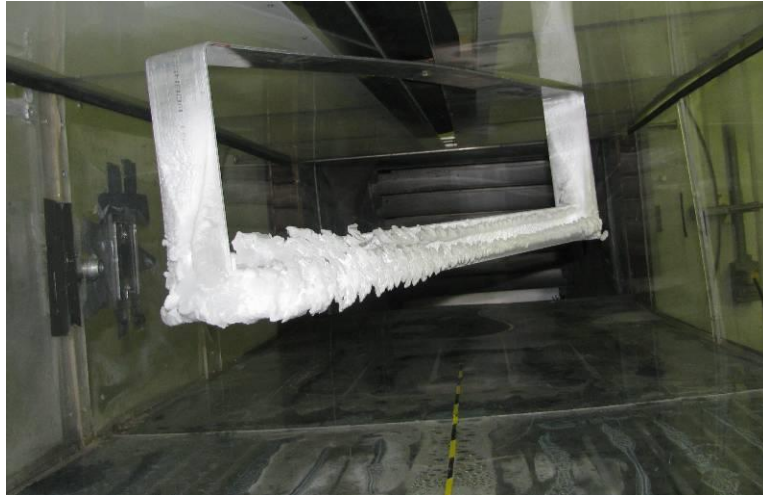
Figure 3-5: Support used for horizontal ice simulation
