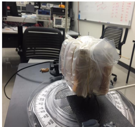
Figure 3.18: Photograph of the test jig showing the rotatable disc, angle dials and biomimetic layer ( covered in plastic)
