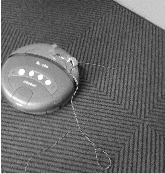
Fig. 1. The robot. An iRobot Roomba vacuum cleaner was used as a platform for the experiments. The whisker was mounted on the front of the robot, angled down to make constant contact with the floor.
