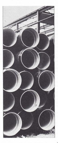
classes: 100, 150, and 200. The higher the number, the thicker the pipe wall. Most utilities use class 150.
