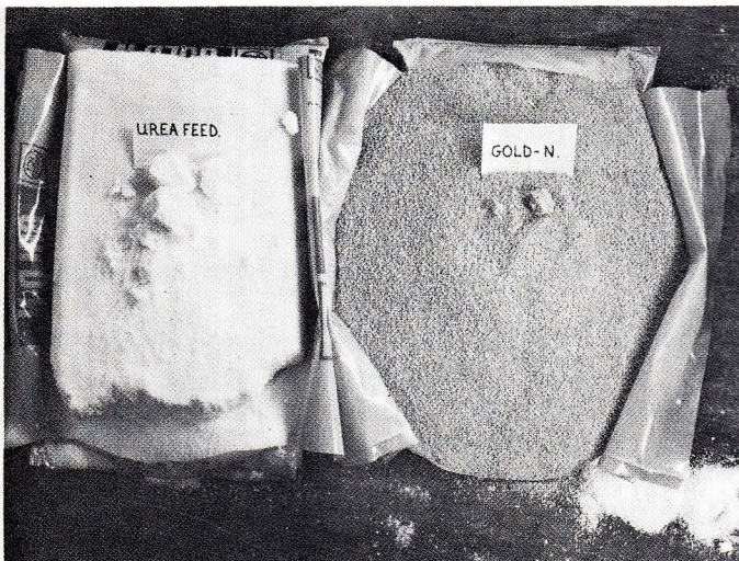
Fig. 2: Caking after storage for two months.
