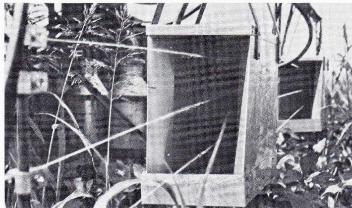
Recirculating sprayer applies “hot” herbicides to tall weeds and captures excess herbicide.
