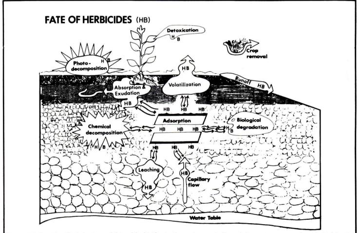
Processes influencing the behavior and fate of herbicides in the environment. Degradation processes are characterized by the splitting of the herbicide (HB) molecule. Transfer processes are characterized by the herbicide (HB) molecules remaining intact.
