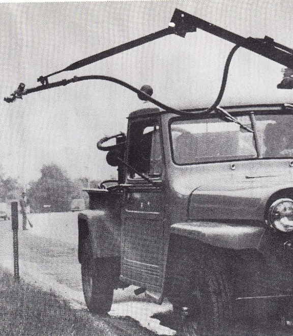
■ APPLICATION by truck-mounted spray boom with two tips for broadcast work or one or two jets for selective spraying. Gauge pressure for spray boom is 50-60 psi.
