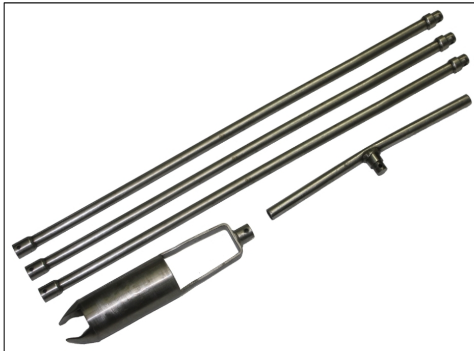
Figure 20. Example of Hand Auger and Extension Rods.
