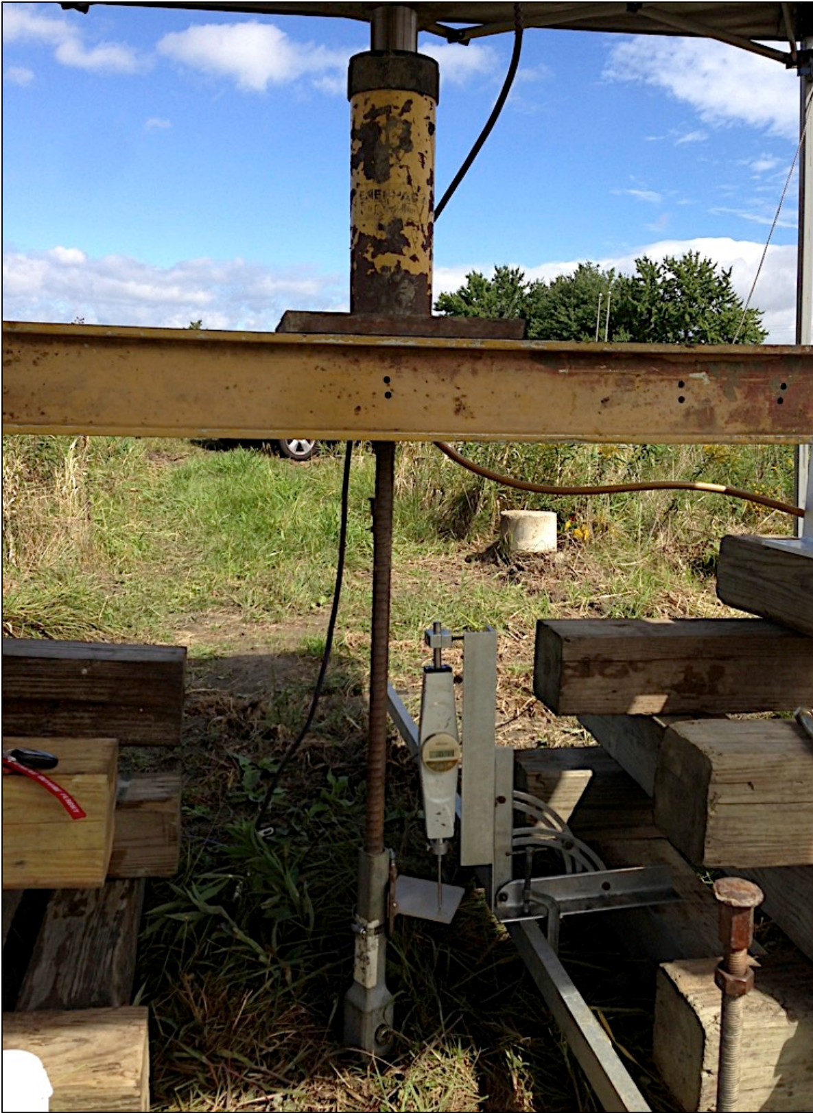
Figure 27. Hydraulic jack and digital displacement gage.
