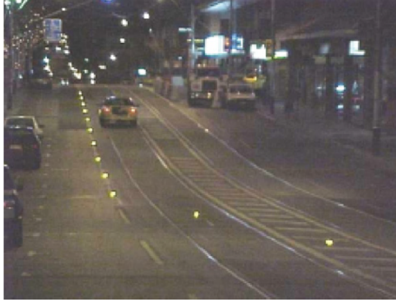
Figure 2.5: Flashing lights of the intermittent bus lane in Melbourne, Australia (Currie and Lai, 2008)
