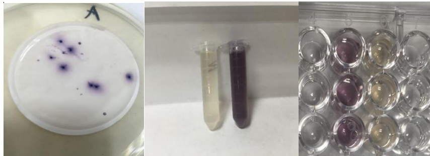
Figure 5.2 Colored signal from the reaction of E.coli strain that overexpressed alkaline phosphatase (ALP E.coli ) with BCIP/NBT substrate on 0.22 \mu\text{m} membrane filter (left); comparison of enzymatic reaction of ALP E.coli with wild type E.coli at the presence of BCIP/NBT substrate in centrifuge tube and 96-well plate, respectively (middle and right).
