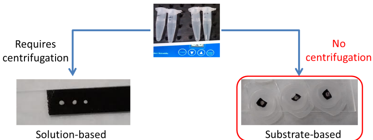
Figure 4.4 Two methods were proposed for using Ag dendrites, one that solely depends on centrifugation while the other largely depended on the use of a double sided tape to stick the Ag dendrites onto the cap of a microcentrifuge tube.
