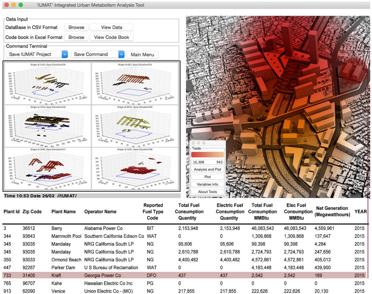
Figure 3.5: Plant selection based on proximity analysis and fuel data from EIA-923 and EIA-860 datasets.
