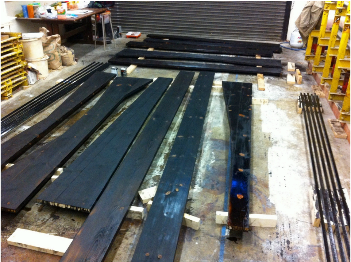
Figure 4.3: Charred woods after applying polyurethane on the surfaces (Image credit by the Author)
