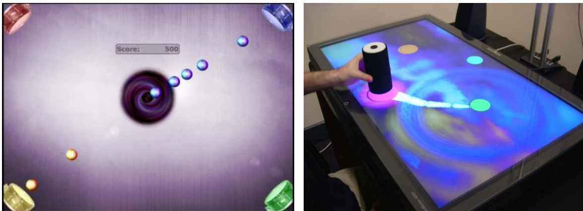
Figure 9. Touchscreen therapy and visual feedback. Left: Mumford augmented feedback [6]. The size of the aura under the solid object and the ripple speed both correspond to patient action and performance. Right: AIRtouch rhythm game [43]. The patient must hit the drums in the corners when the balls from the center reach them.
