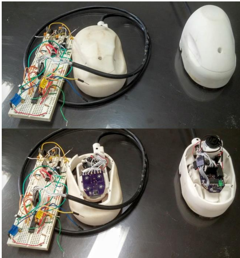
Figure 36. Comparison between the two prototype iterations. The first iteration is on the left with its outboard electronics shown, and the current iteration is on the right.
