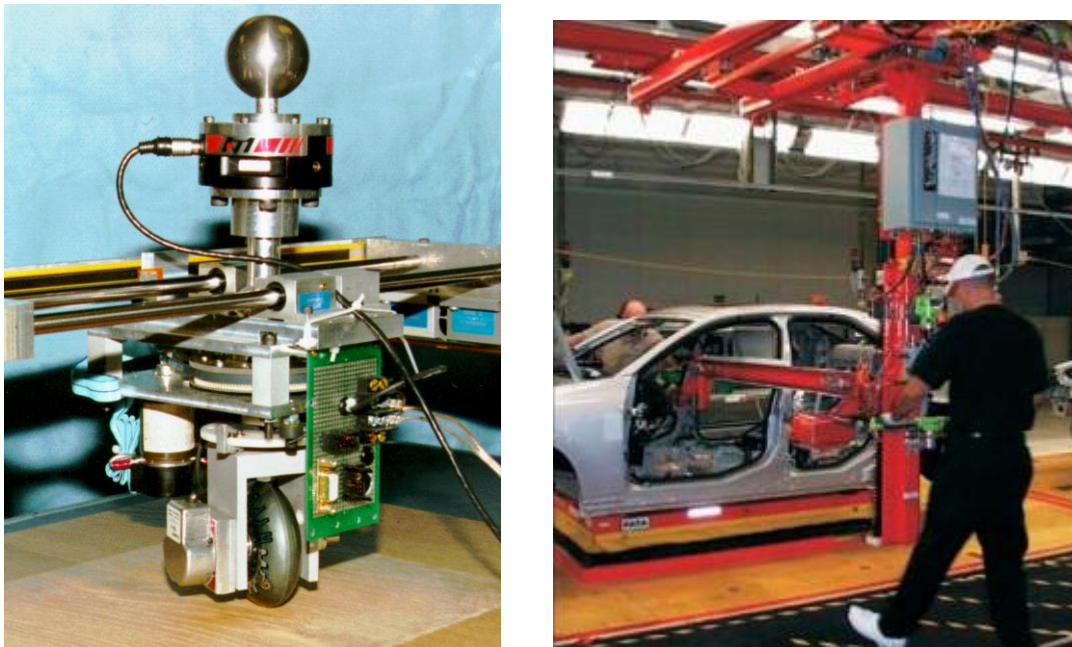
Figure 4. Cobot platforms. Left: The Cobot unicycle. Right: Car cockpit installation assisted by assembly scale Cobot. Produced by commercial offshoot Cobotics. [33]
