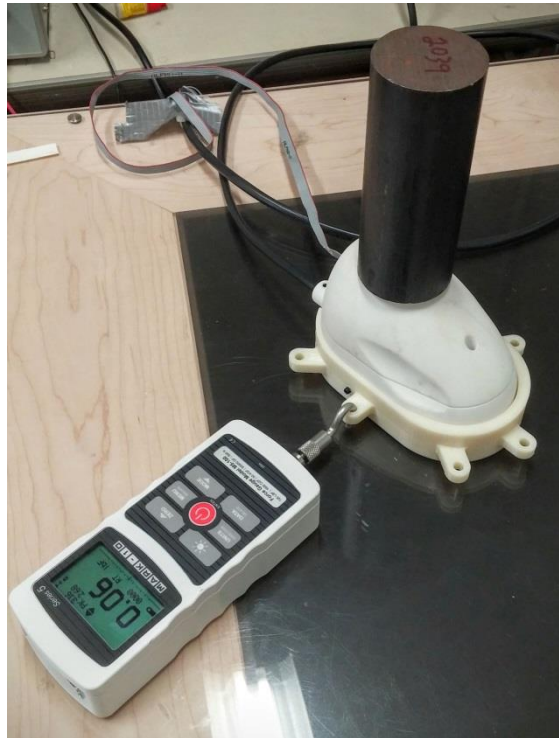
Figure 31. Friction and force sensor validation test setup. The prototype is shown in its test fixture and under its 20 N load weight.
