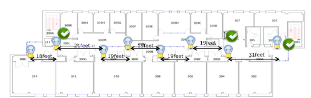
Figure 51 Deploy layout in Knowles Engineering building
