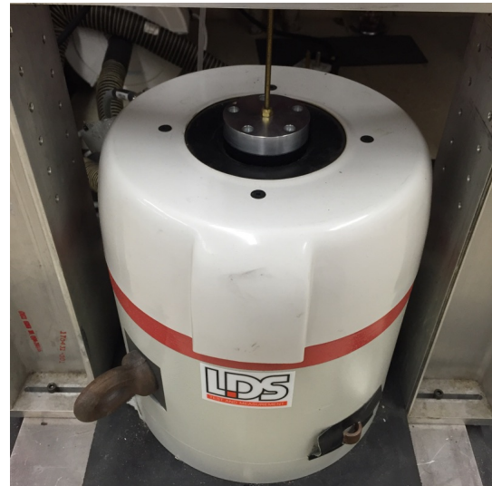
(b) View of the base of the shaker. One can see the brass rod that leads up to the air bearing.
