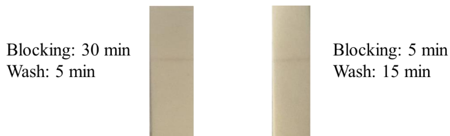
Fig. 5.5. Effect of blocking time of nitrocellulose with 1% non-fat dried milk and washing time with 1 x PBS.
