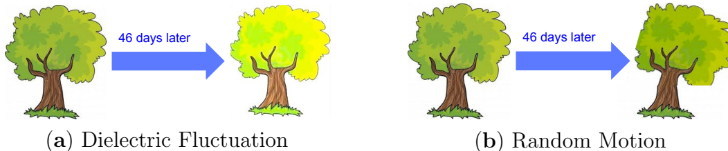
Figure 1.4: The temporal decorrelation effects due to dielectric change and random motion of the volume scatterers within a repeat period of 46 days.
