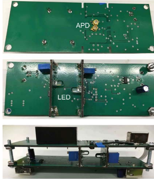
Fig. 17 The assembled second version discrete-component fluorimeter
