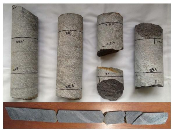
Figure 40: Core samples from hydraulically active portion of well selected for testing using core scanning with Geotek MSCL and ITRAX<sup>TM</sup> XRF.
