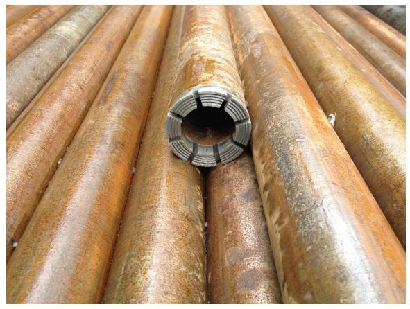
Figure 37: Drilling rods and HQ-sized (96 millimeter outer and 63.5 millimeter inner diameter) rock coring bit used to drill borehole MFS-1 at the MacLeish Field Station in Whately, MA.
