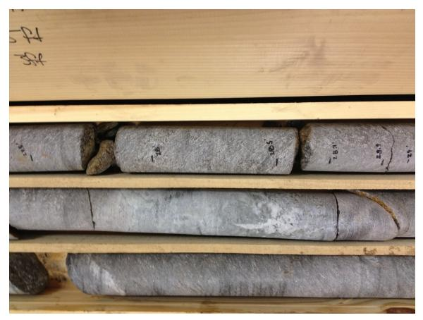
Figure 38: Core from the interval of 8.2 to 9.1 meters (27 to 30 feet) below ground surface. Iron staining was identified on the fracture surfaces in this interval and downhole geophysical testing supported that advective flow into the well is likely occurring along one of the fractures in this zone. Note the broken zone between 8.4 and 8.5 meters (27.5 and 28 feet) below ground surface with significant iron staining on the broken surfaces of the rock.
