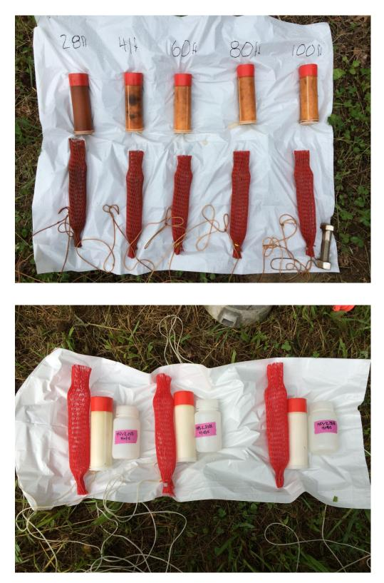
Figure 17: Iron staining on the RPP samples after two years deployed in Well MFS-1 (top) and lack of iron staining on RPP samplers deployed in MFS-2 (bottom) over the same period.
