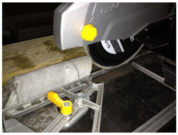
Figure 39: Rock saw using water and diamond blade to cut core samples along the long axis for geochemical testing.
