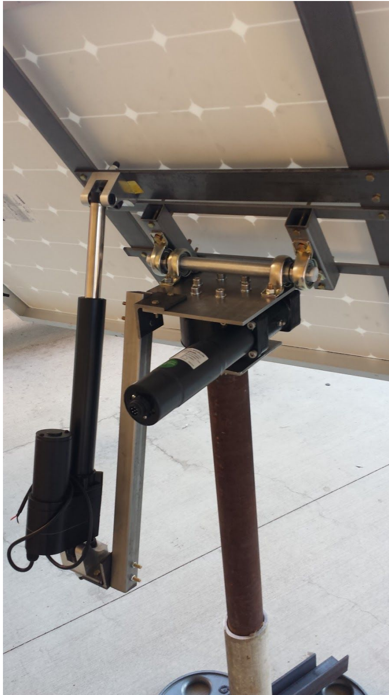
Figure 19. Rear view of assembled tracking mount.
