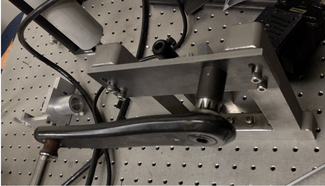
Figure 16. The final cantilevered spindle mount fixture shown with a crank arm installed without the bottom bracket.
