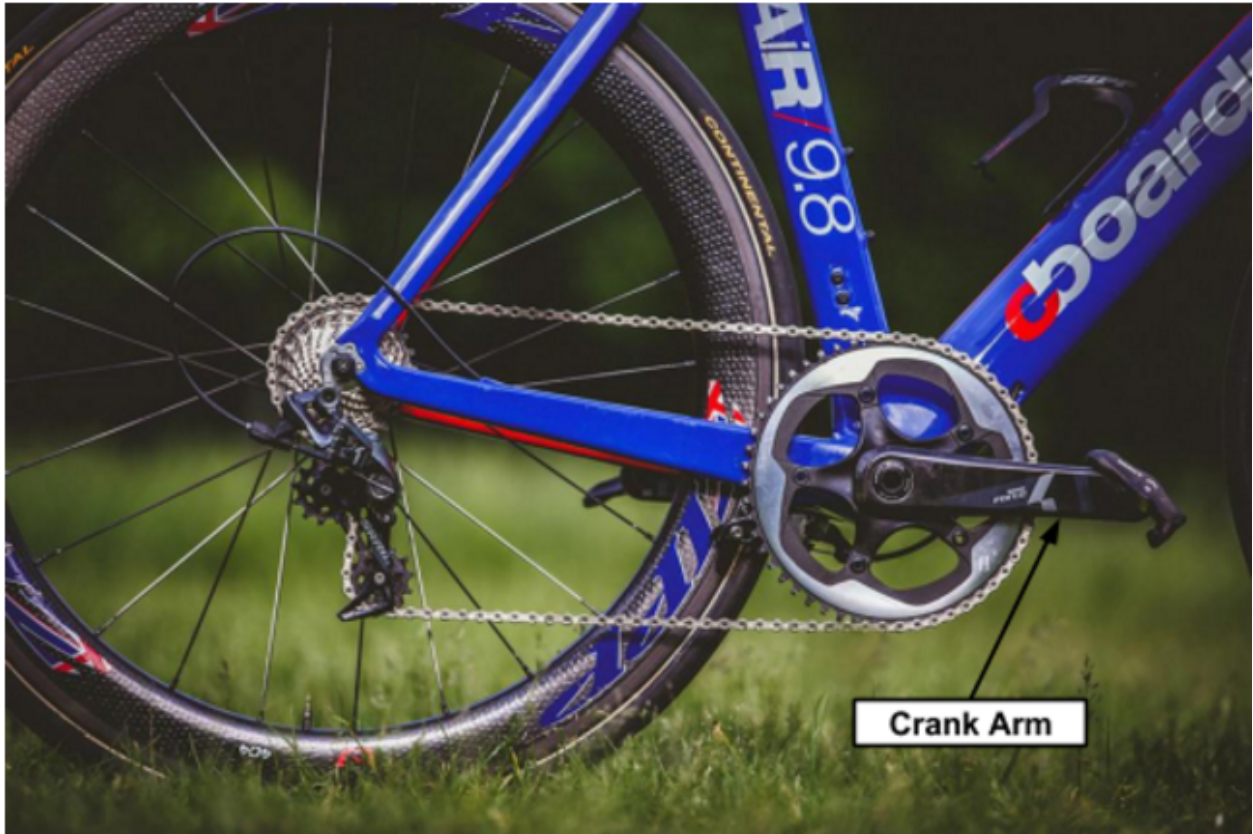
Figure 3. Crank arm location on a bicycle. A crank arm links the pedal to the crank, transferring power as the rider pedals [2].
