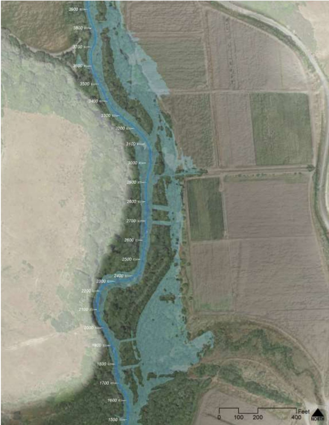
Figure 10. HEC RAS model results for the bankfull event showing potential inundation (shaded blue) through the proposed levee breaches.
