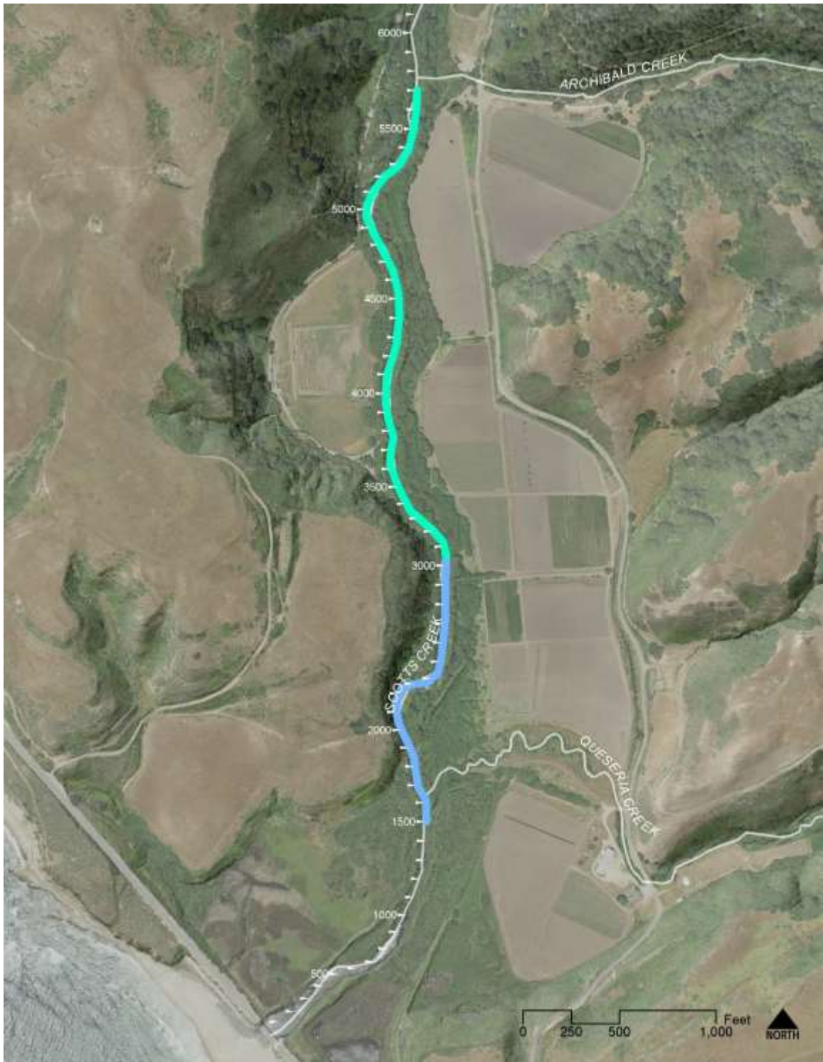
Figure 9. Project reaches with river stationing in feet upstream from the CA-1 bridge. Blue denotes Phase I, cyan Phase II. Stationing is offset by approximately -100 feet compared to stationing shown in the 100% design drawings.
