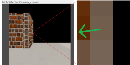
Figure 3.8: V-REP gradient for one pixel. Gradient vector in green.
