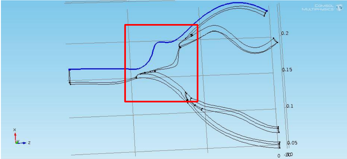
Figure 3.13: Blue line depicting the outer edge of the vessel from which the shear stress data was extracted
