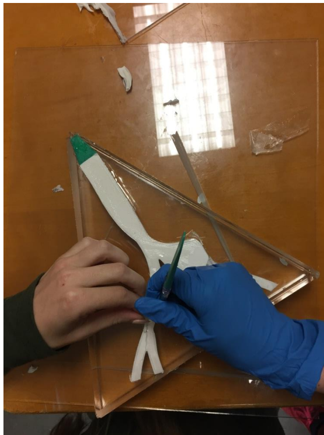
Figure 2.8: Removal of excess PDMS around the printed part
