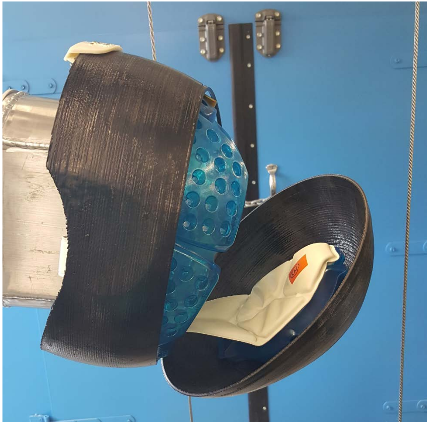
Figure 32. Control helmet after being destroyed by drop testing
