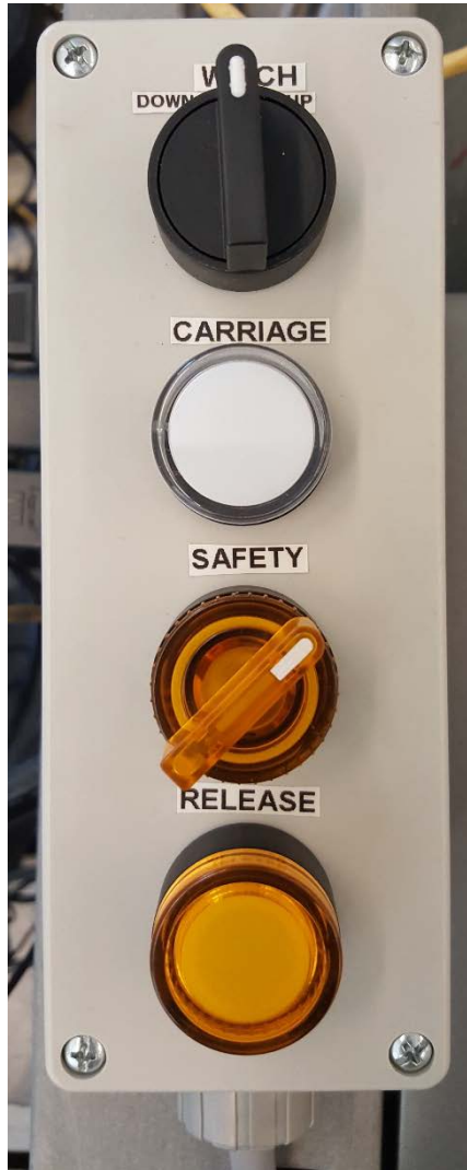
Figure 27. The drop tower control pendant
