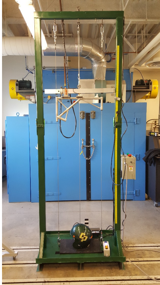
Figure 15. The NOCSAE style drop tower designed for Cal Poly
