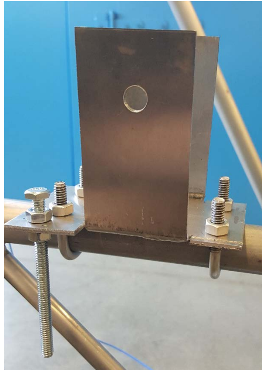
Figure 23. The safety bracket attached to the carriage
