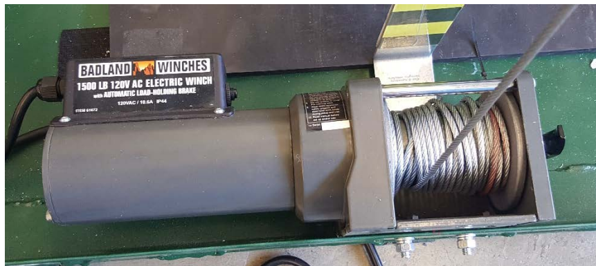
Figure 21. Harbor Freight winch responsible for positioning of lift bar
