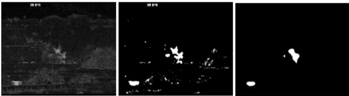
Figure 45 - Results of Difference Image Method with Delta = 5sec. Source: Garges Figure 26
