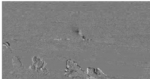
Figure 3 - The 7th PC image showing the traces of the fire plume and moving tree branches against a mostly flat background. Source: SPIE 2011
