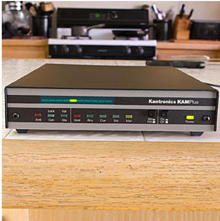
Figure 3.1. Image of the Kantronics KAM Plus TNC [37].
