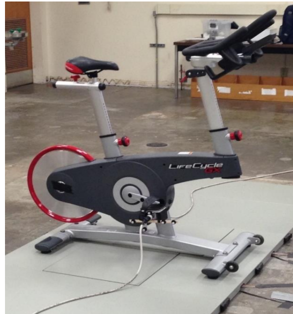
Figure 2.6 Upright stationary bicycle location and set up for biomechanics experiments.
