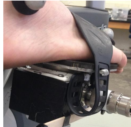
Figure 2.8 Pedal strap is bent under itself to avoid blocking a marker.
