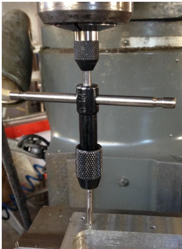
Figure C.5 Thread tapping set up using vertical milling machine.
