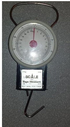
Figure 108: Force gauge used in the pull testing.
