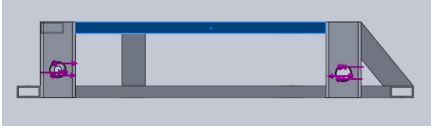
Figure 142: Tread tension and bearing loading conditions.
