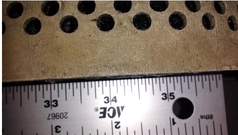
Figure 115: Angular misalignment of the tensioner wheel on the right side of the vehicle.
