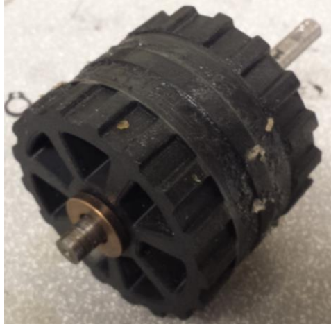
Figure 78: The drive wheel pressed onto its shaft.
