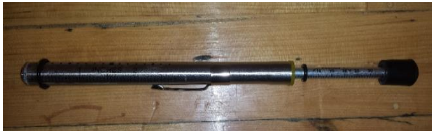
Figure 118: The force gauge used to determine the tread tension.
