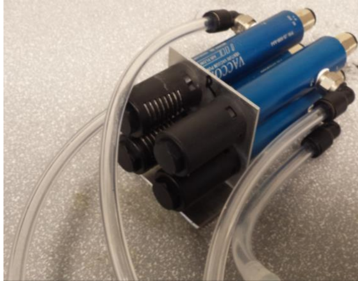
Figure 66: Venturi mounting bracket with the venturis installed.
