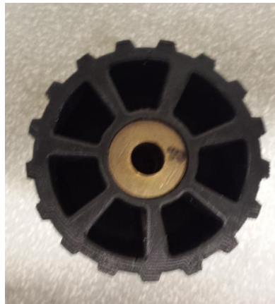
Figure 85: Tensioner wheel with the bushings in place.
