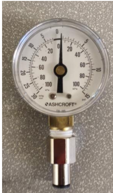
Figure 97: Vacuum gauge used during the pressure system testing.
