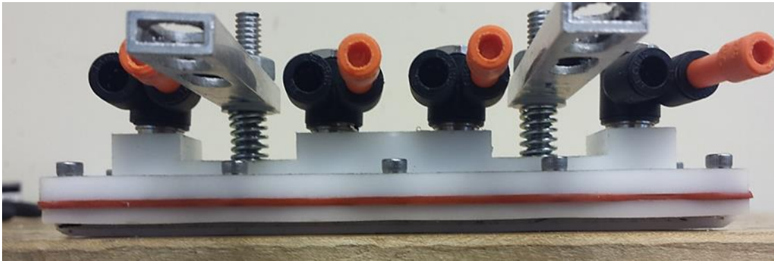
Figure 70: The bending seen in the right lower manifold half.
