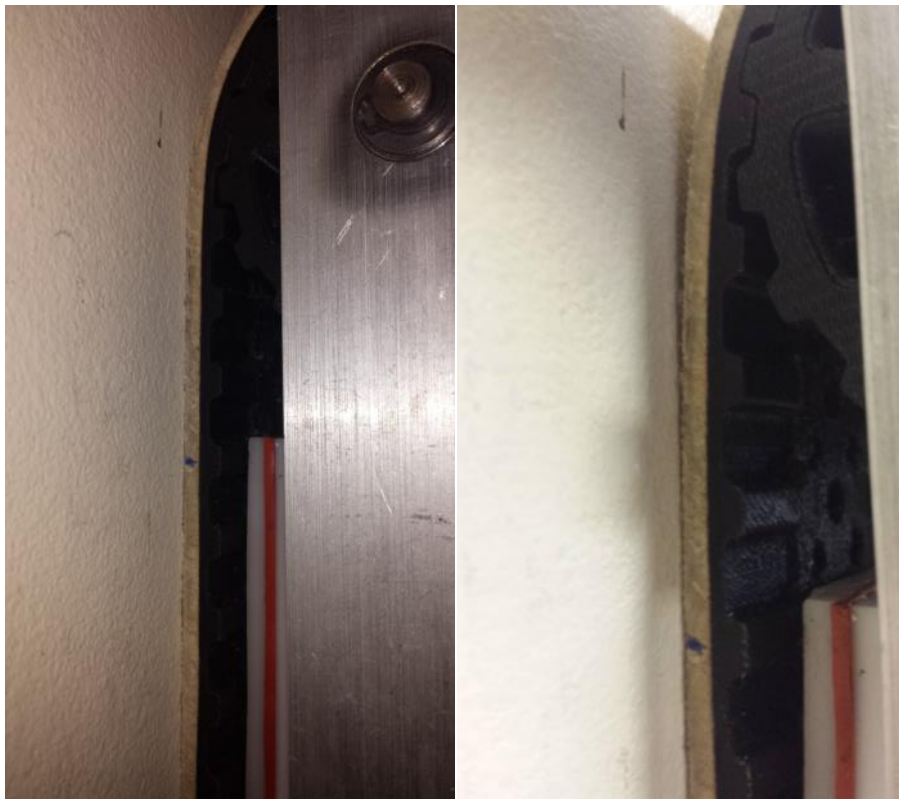
Figure 105: (Left) the right tread after it was pressed onto the wall. (Right) the right tread before it was pressed onto the wall.
