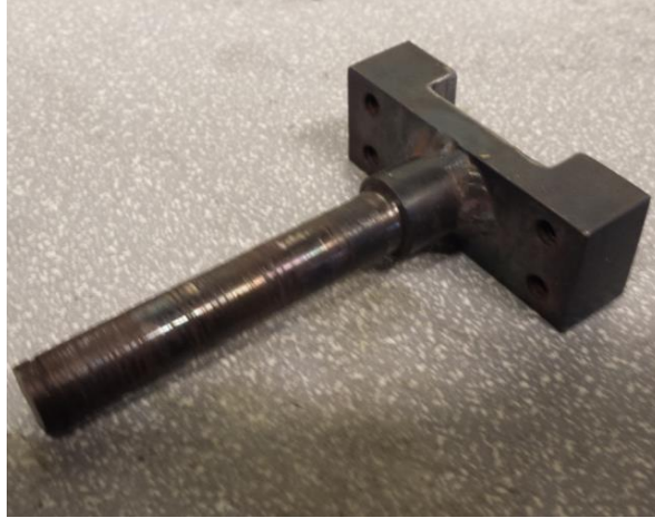
Figure 86: Tensioner shaft after it was welded to the exterior clamp half.
