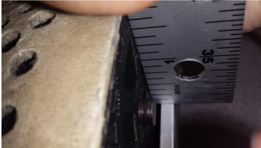
Figure 117: Angular misalignment between the brace and the tensioner wheel on the right side of the vehicle.
