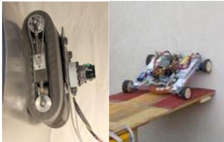
Figure 8: (Left) The ICM Climber which employs an active vacuum adhesion system [21]. (Right) The Alicia VTX robot which employs a vortex system [22].
