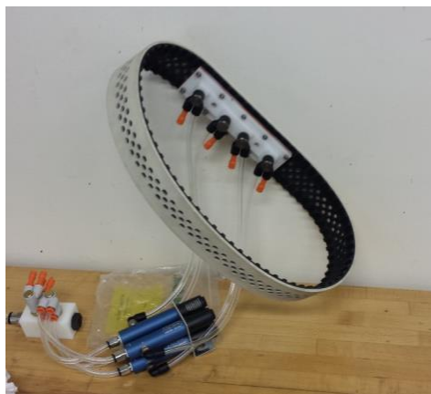
Figure 120: A tread being adhered to the wall with a manifold.
