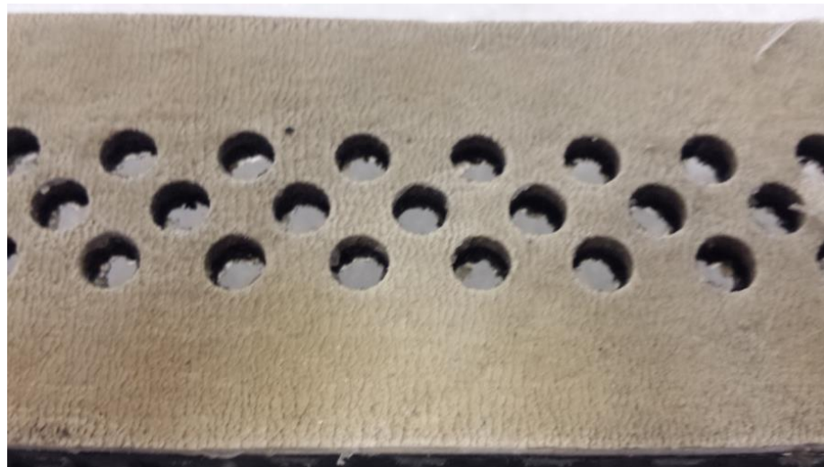
Figure 91: Tread backing after the silicone sealant was applied.
