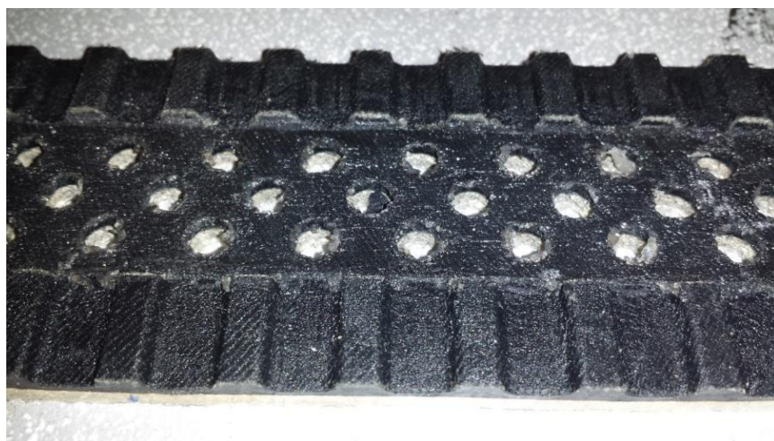
Figure 89: Low friction fabric after the application of the silicone sealant.
