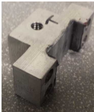
Figure 84: Interior clamp half.
