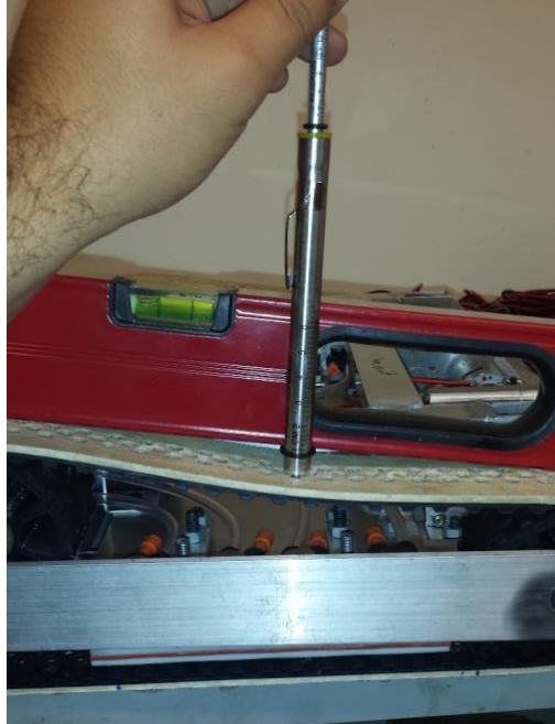
Figure 119: The tension in the left tread being measured.
