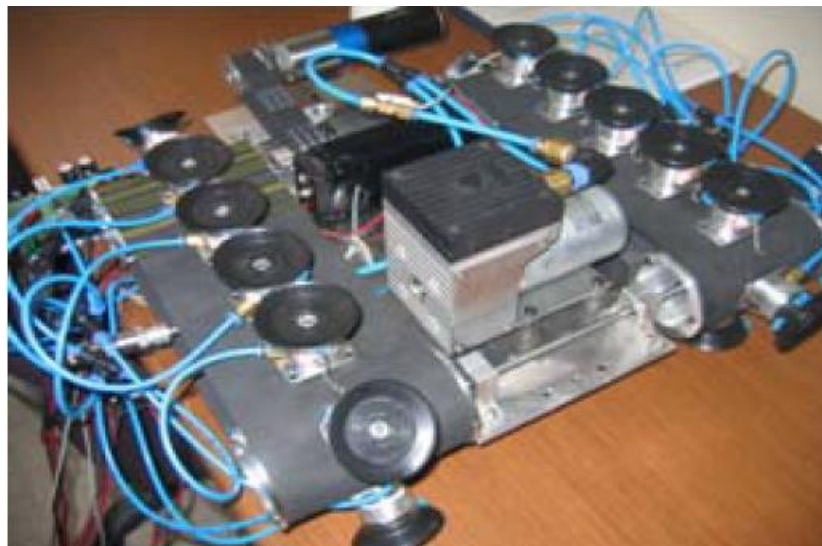
Figure 13: A climbing robot which uses active suction cups attached to a continuous tread [8].
