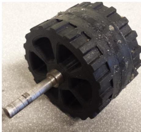
Figure 77: The idler wheel pressed onto its shaft.
