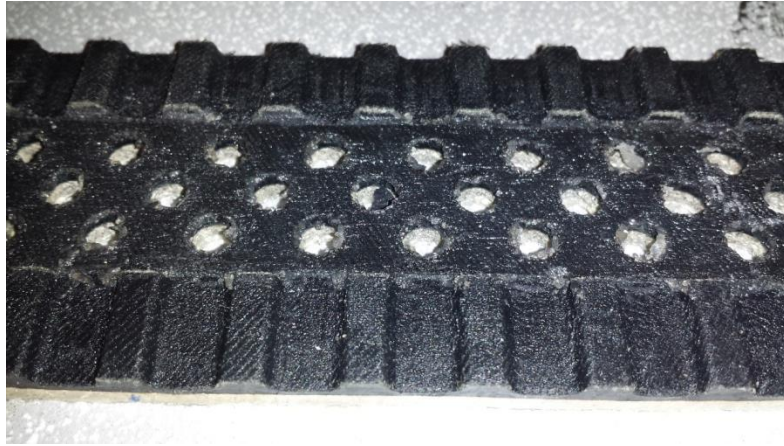
Figure 124: Low friction fabric after the silicone sealant had been applied.
