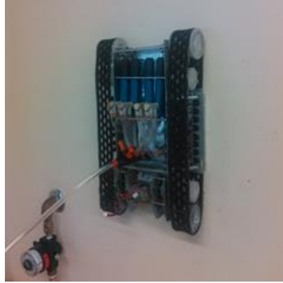
Figure 16: Proof of concept model adhering to a vertical surface.
