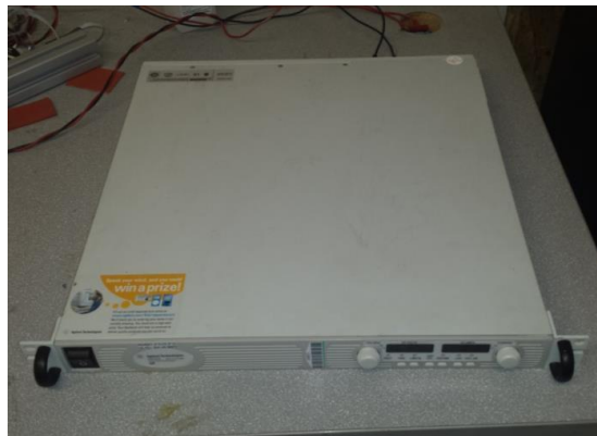
Figure 19: Agilent N5747A power supply used to power the vehicle.
