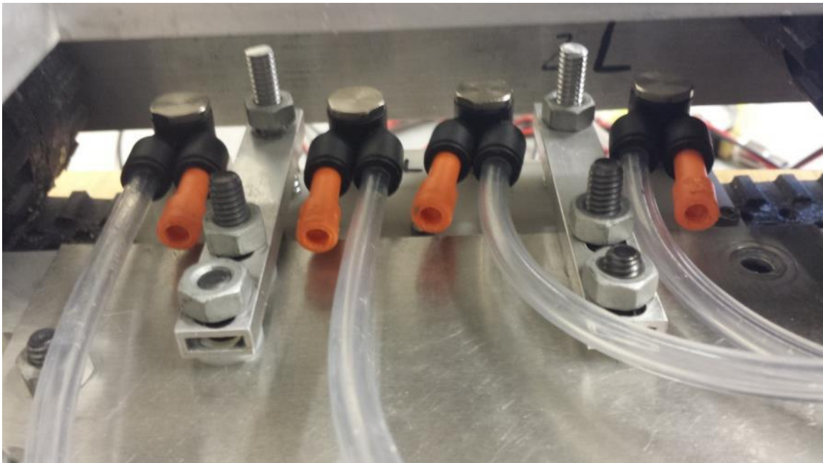
Figure 95: Manifolds from the inside of the vehicle.
