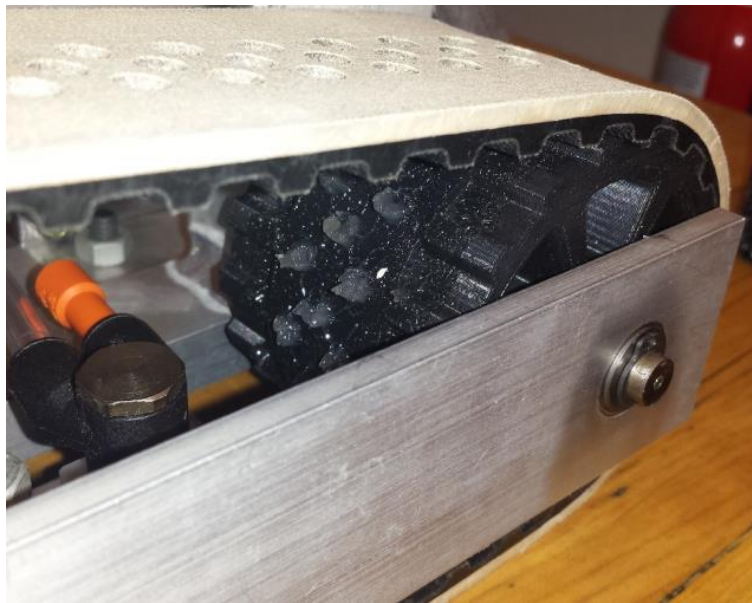
Figure 123: Grease spikes which were squeezed into the tread holes during operation.
