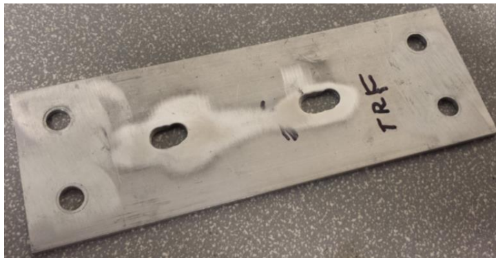
Figure 63: Right side motor mounting plate. Note the slots cut so the motor could be adjusted.
