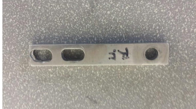
Figure 73: One of the manifold mounting struts.
