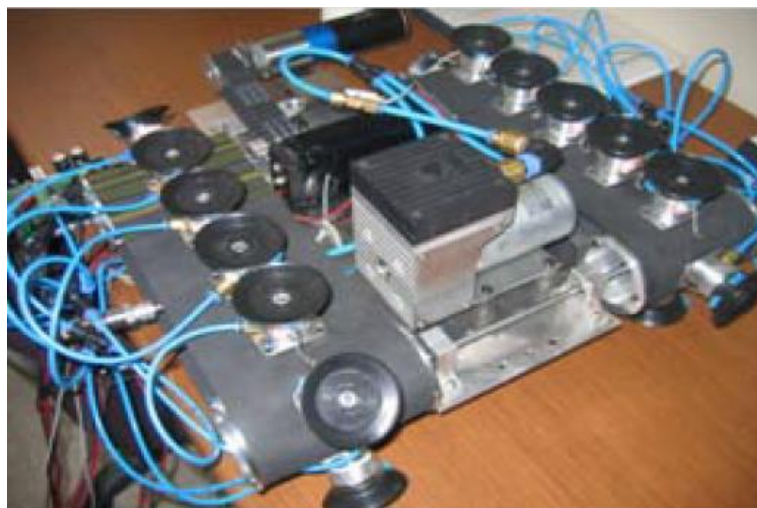
Figure 3: An example of a treaded wall climbing robot from [8].
