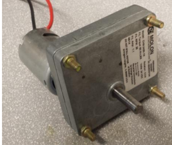
Figure 18: Molon motor chosen for the vehicle.
