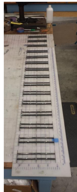
Figure 4.4.6: All 15 completed internal structures for wing design
