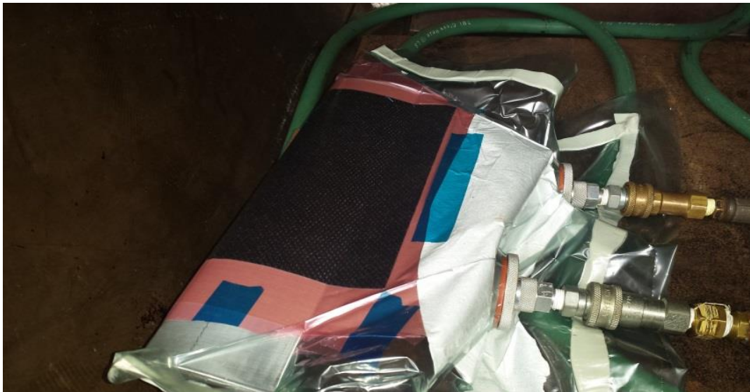
Figure 4.2.3: Wing skin in vacuum bag just before curing in autoclave
