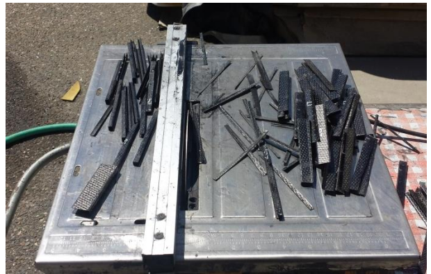
Figure 4.3.4: Cutting process used to trim spars down to size
