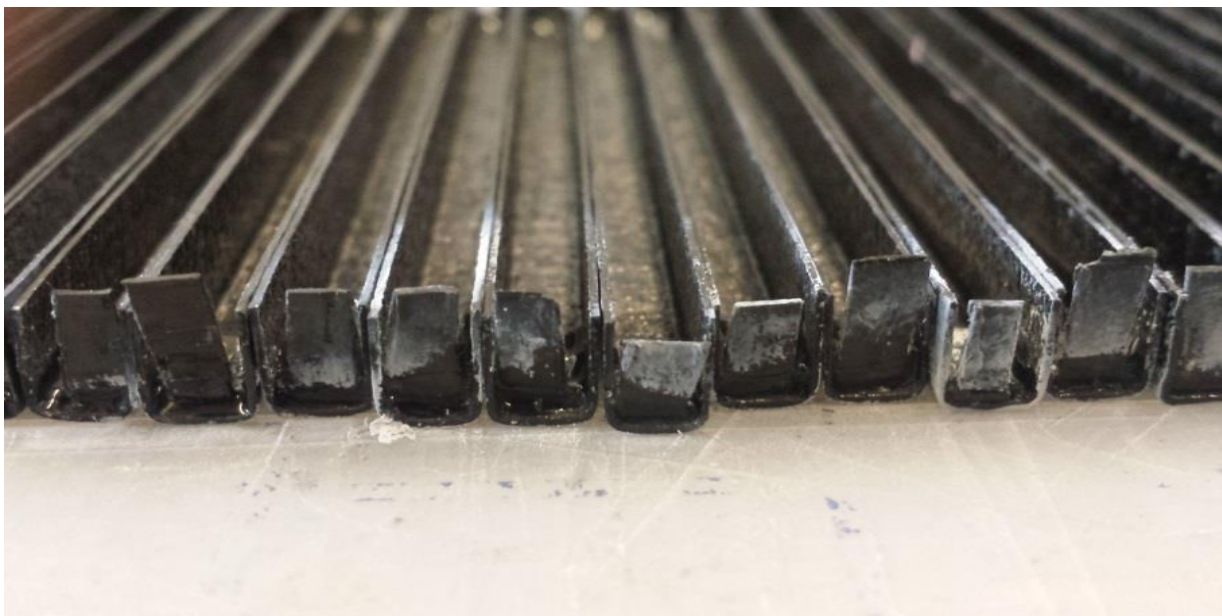
Figure 4.3.5: Row of leading edge spars with L-brackets attached using super glue
