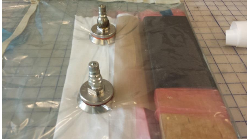
Figure 4.2.2: Vacuum bag of experimental cure to determine validity of proposed manufacturing method of the wing skin
