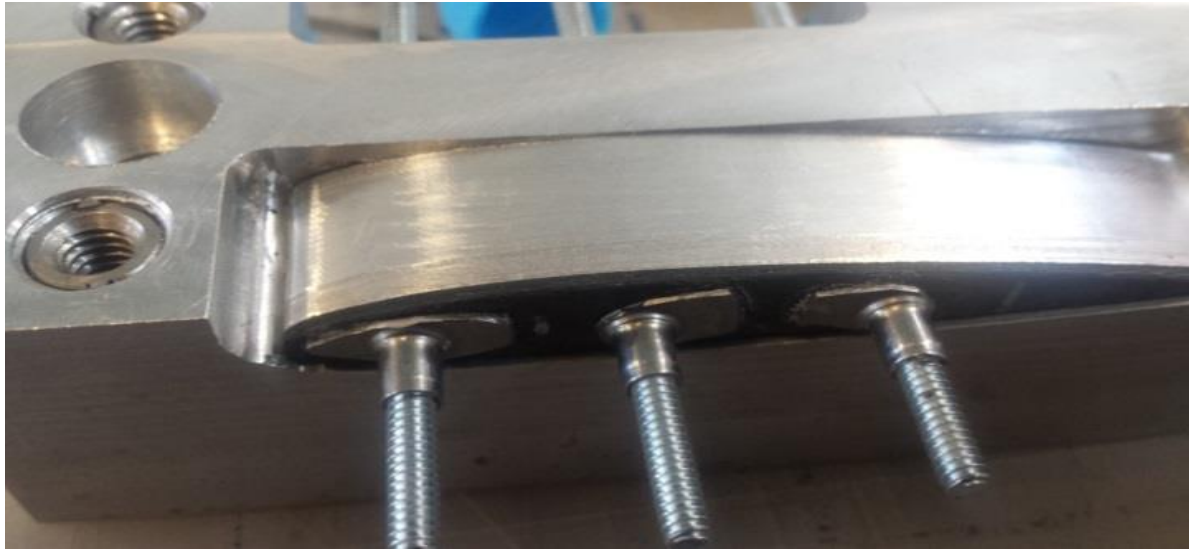
Figure 4.3.7: Method used to ensure that the weld-nuts aligned with the mounting rib for best possible fit
