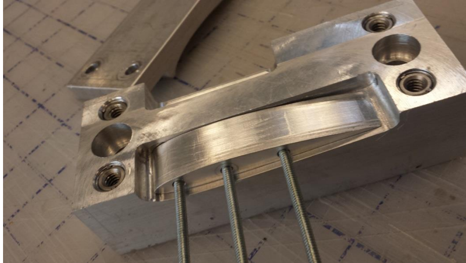
Figure 3.4.2: View of how aluminum plug and screws fit onto mount
