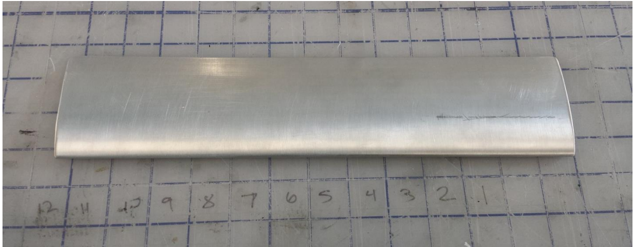
Figure 4.2.4: Wing skin mold after sanding and polishing
