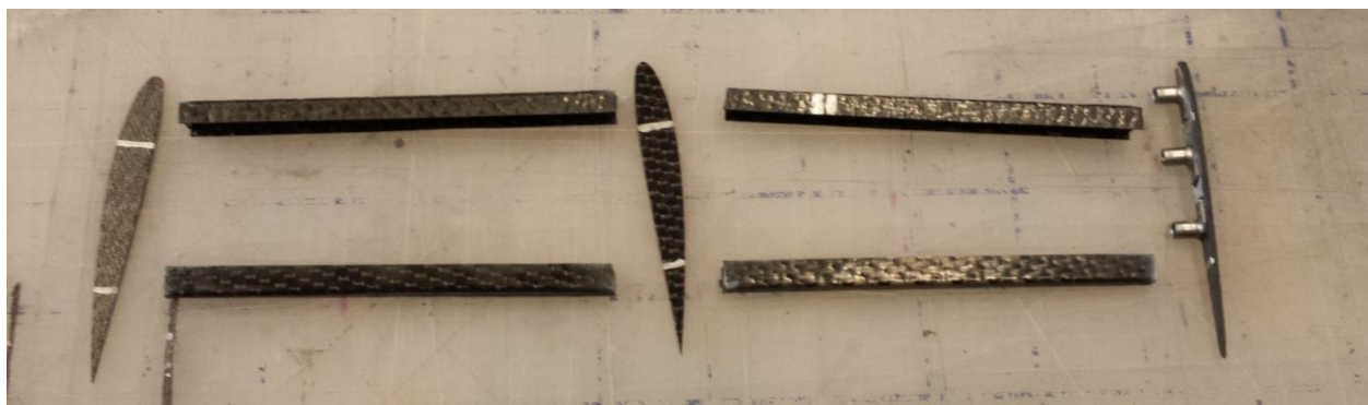
Figure 4.4.2: Layout of how internal structure will be pieced together
