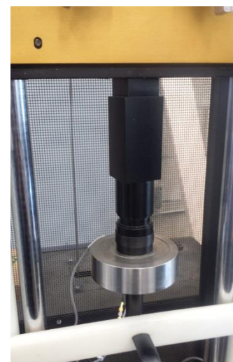
Figure 2.2.2: Original Fixturing of Load Cell
