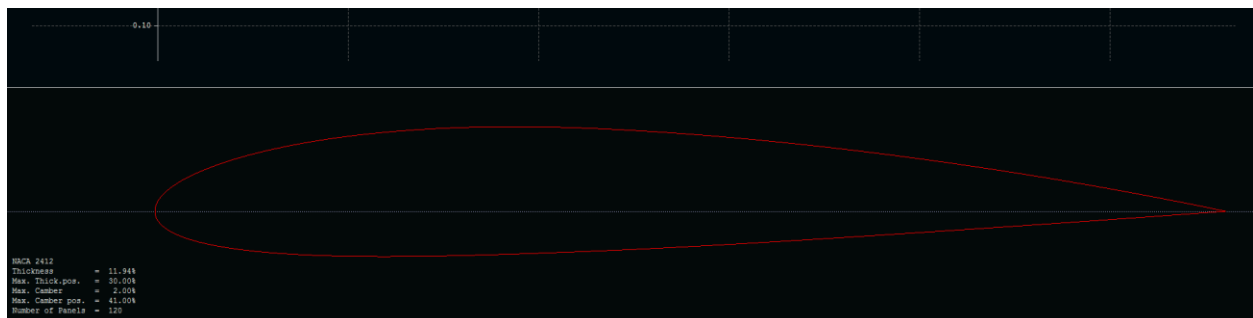
Figure 6.2.1: Creation of NACA 2412 airfoil X and Y coordinates in XFLR5 for use in Abaqus
