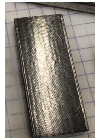
Figure 4.2.1: Successful test of manufacturing method of wing skin with carbon being removed from mold with ease
