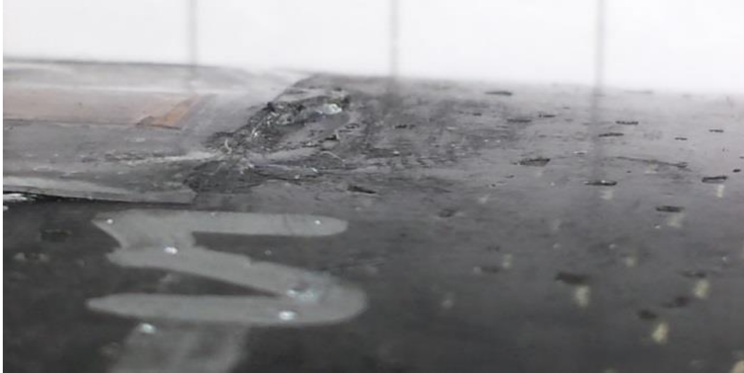
Figure 5.3.4: Close up of impact damage sustained by wing
