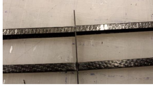
Figure 4.4.5: Top-down view of middle rib after having both sets of spars glued in place
