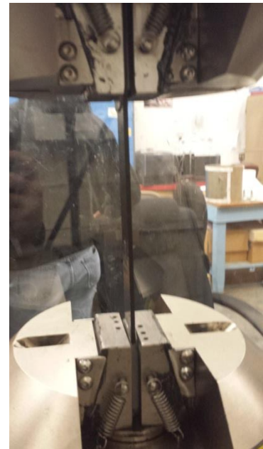
Figure 2.1.1: ASTM D3039 Tensile Testing of Carbon Fiber Specimen
