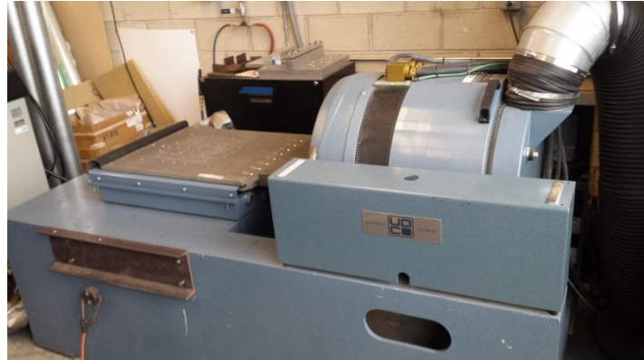
Figure 2.3.1: Unholtz-Dickie Shaker Table System used for testing set to do horizontal excitation
