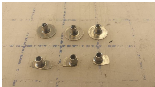
Figure 4.3.6: Original size of weld-nuts and trimmed base of weld-nuts for gluing to mounting rib
