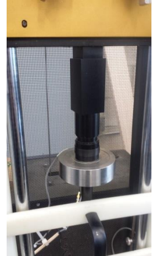
Figure 3.3.2: Original constraining of load cell showing outer cylinder of load cell being unconstrained
