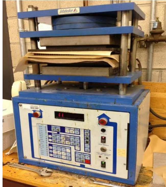
Figure 1.3.2: Heat press used to cure composite materials in the Cal Poly aerospace composites lab
