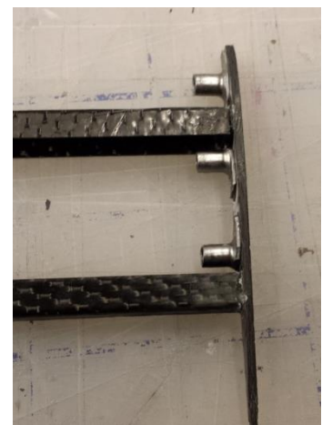
Figure 4.4.4: Mount rib with both leading and trailing edge spars glued in place
