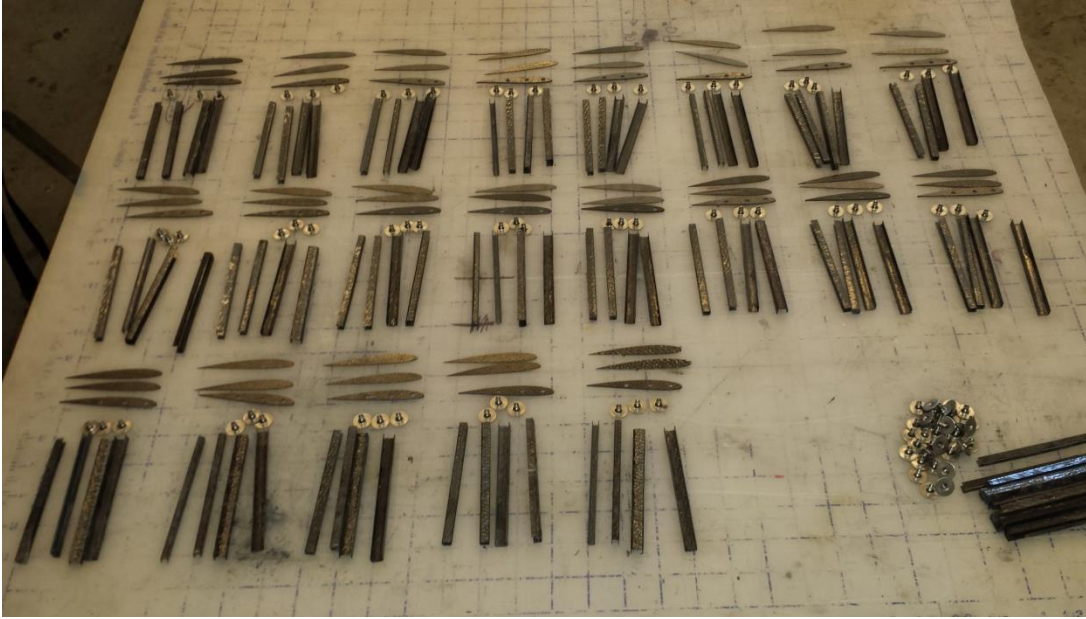
Figure 4.4.1: Layout of wing specimen sets including ribs, spars, and weld-nuts
