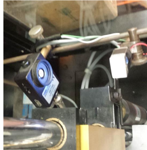
Figure 2.2.1: Si Detector and laser used to measure impact velocity
