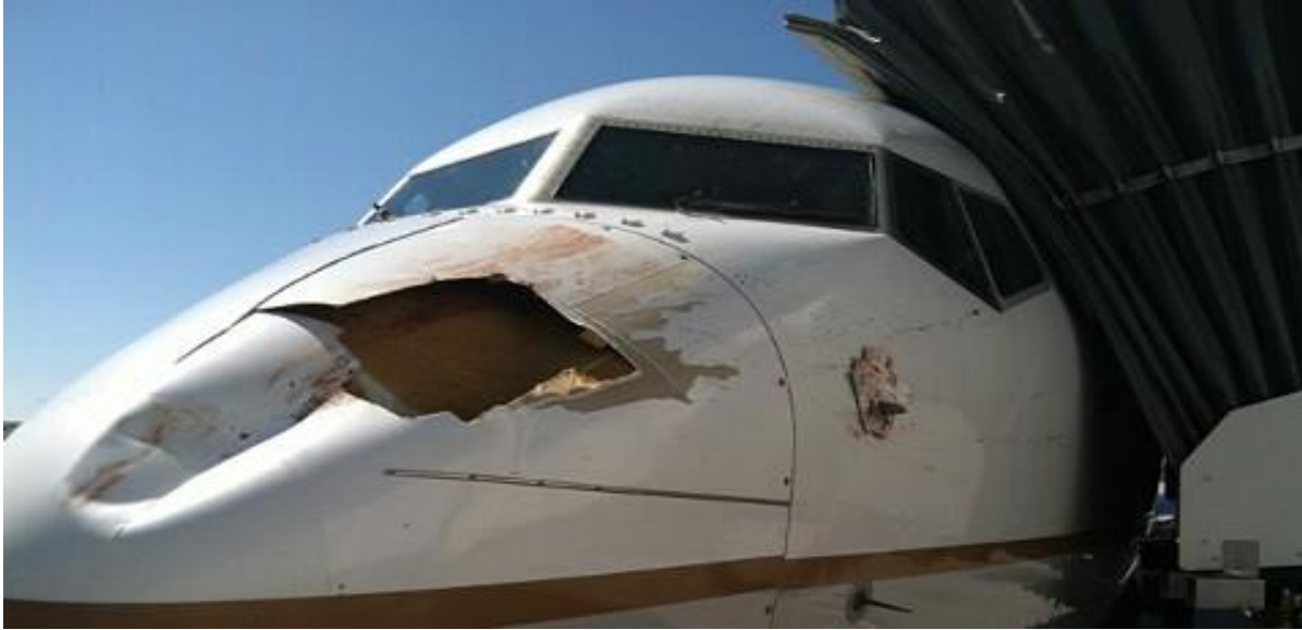
Figure 1.4.1: Aftermath of a bird strike to the nose of an aircraft
