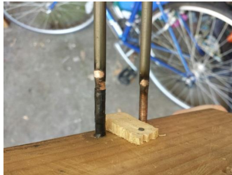
Figure 60: Minimal Damage Done to Copper Tungsten Rails
