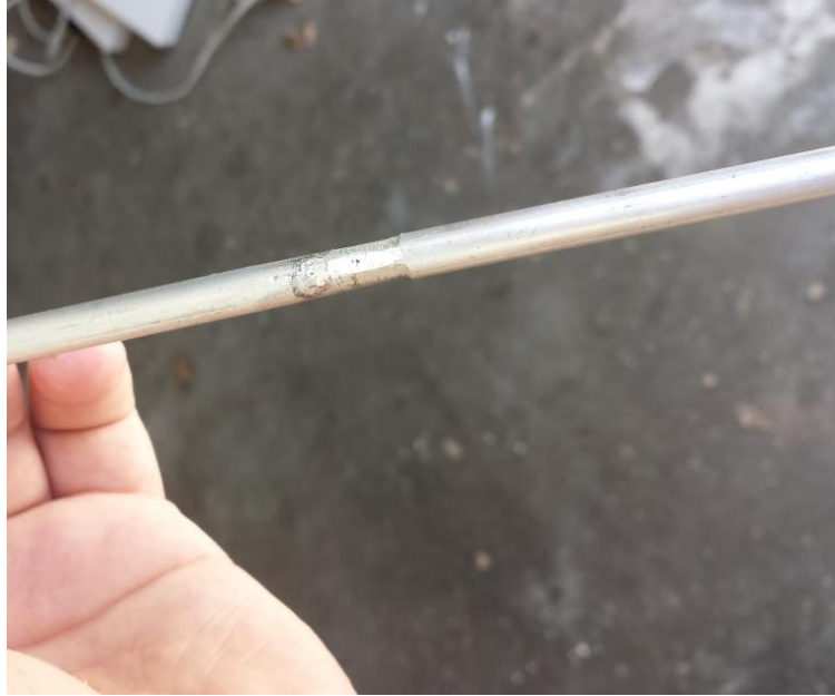
Figure 51: Erosion of Rails After Test #1 (17.5KA for approximately 35 \mu s)
