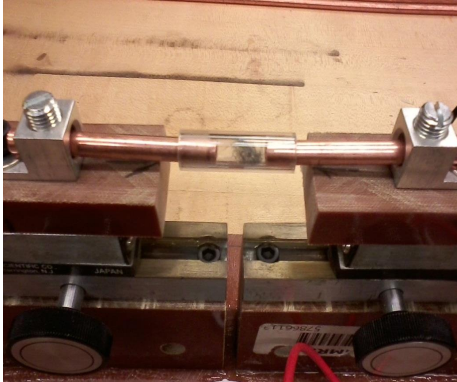
Figure 4-4: UL Specifies Using Steel Wool to Help Initiate Arcing
