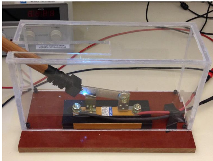
Figure 4-6: Knife Switch Arc Generator Design
