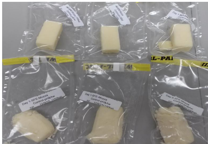
Figure 3-3: Appearance of Mozzarella Cheese before (top) and after SFE (bottom) Treatment at 150 Bar with 50°C for 30 min
