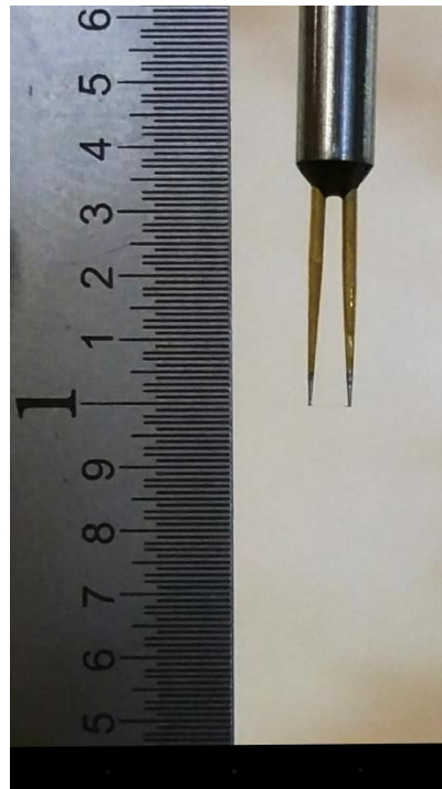
Figure 2.7 Image used to determine hot wire distance from nozzle outlet
