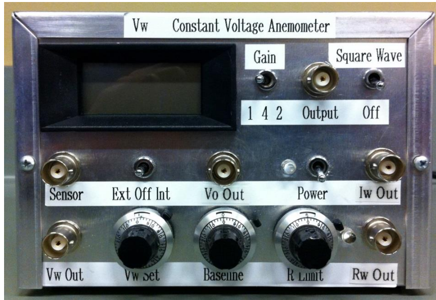
Figure 2.1 CVA I system built for Cal Poly BLDS [1]
