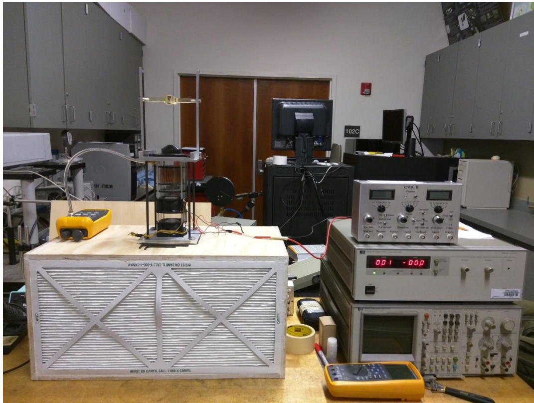
Figure 5.3 Test set-up for calibration and centerline measurements with filter box
