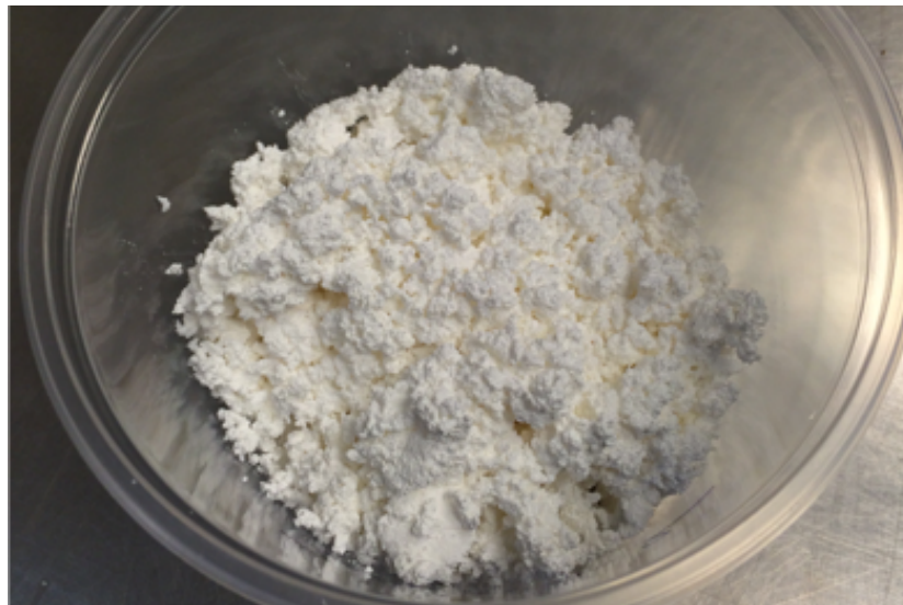
Figure 3-10: Down-Selected B-1000 Binder and Zirconia Mixture
