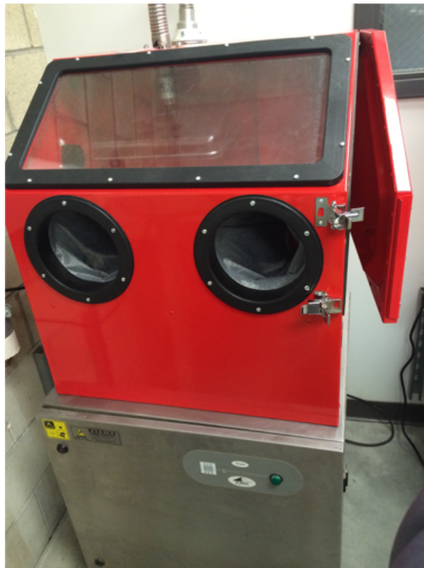
Figure 3-2: Air Filtration Chamber
