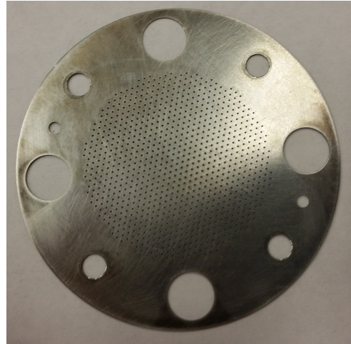
(b) MiXI Acceleration Grid
