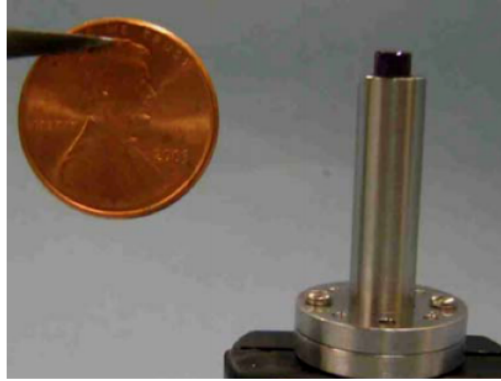
Figure 2.2: Miniature Internal Conduction Hollow Cathode [42]
