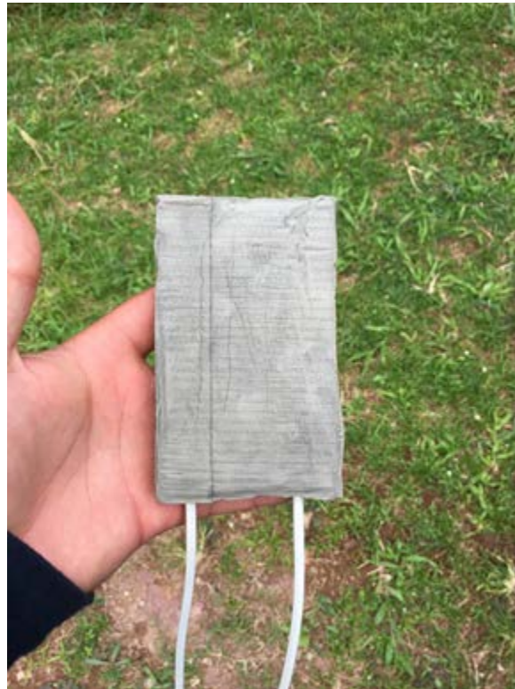
Figure 7.2: Dried heating element
