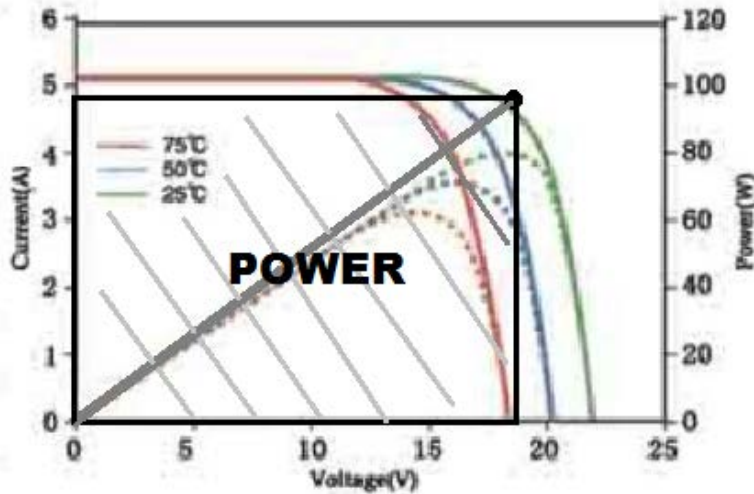
Figure 4.7: Power curve of PV panel
