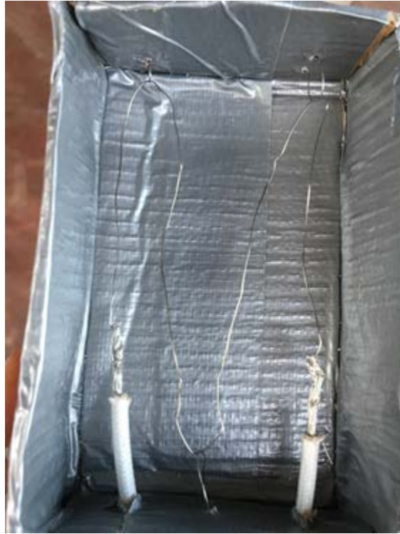
Figure 7.1: Ni-chrome wire configuration of the heating element
