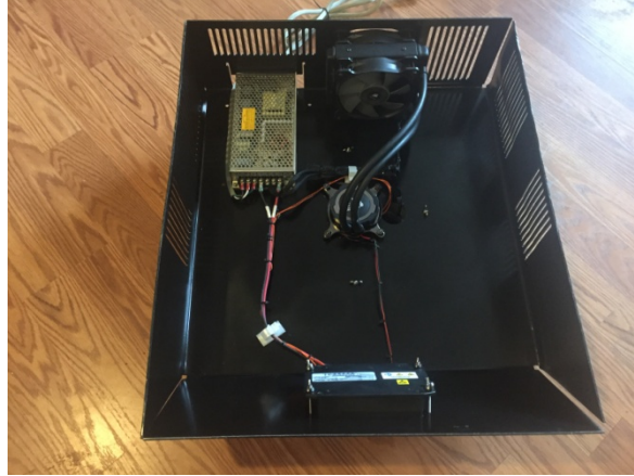
Figure 13. The underside of the new AMA unit prototype housing showing the internal components and the wirings.
