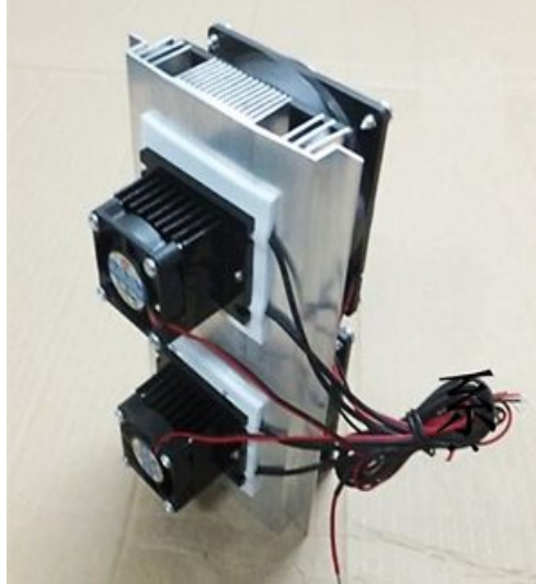
Figure 18. An example of commercially available Peltier assembly. The side facing front shows the smaller cold radiator/sink with fans while the side facing away has much larger heat radiator/sink with fans that can compensate for Peltier cooler's rather low efficiency.
