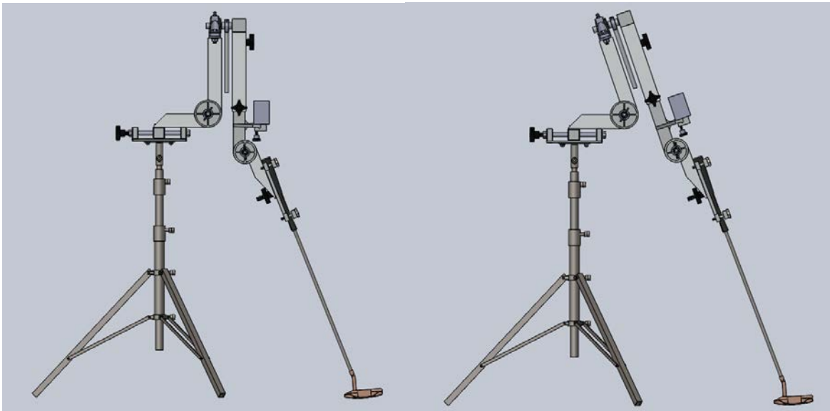
Figure 5.4. Swing plane adjusts to include 90-degree (left) and 71-degree (right) strokes, and anything in between.
