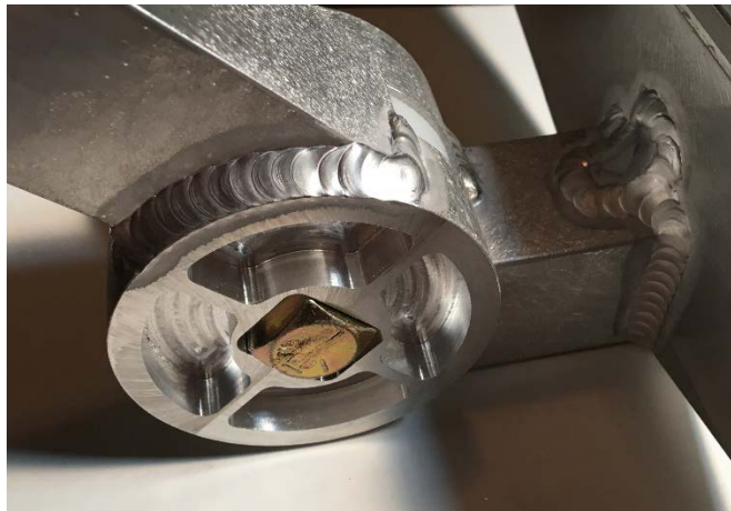
Figure 7.3. This joint piece is one example of the use of CNC machining (for the quarter-circle pockets as well as the rectangular pocket to hold the bolt).
