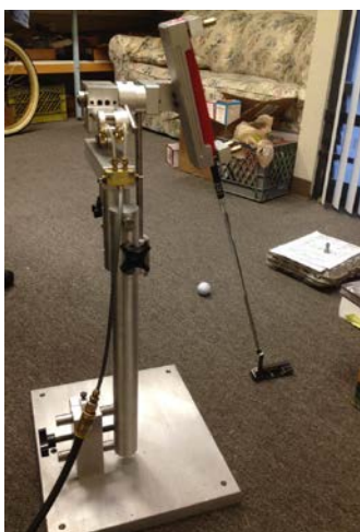
Figure 2.10. Kronos Golf putter testing robot.
