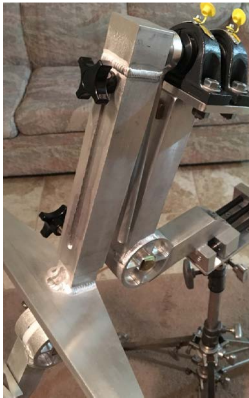
Figure 7.1. Overview of tubing layout in final machine structure. Note that the smaller down tube is concealed inside the larger down tube (with the black knobs) in this photo.
