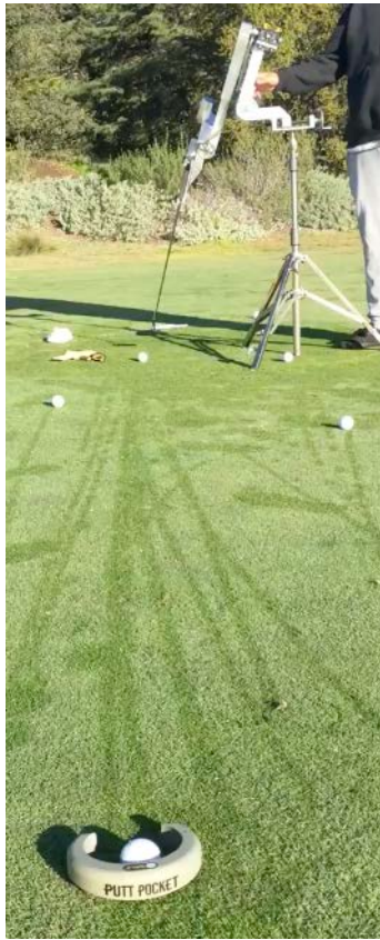
Figure 8.2 Accuracy test on the Cal Poly putting green with putting gate shown.
