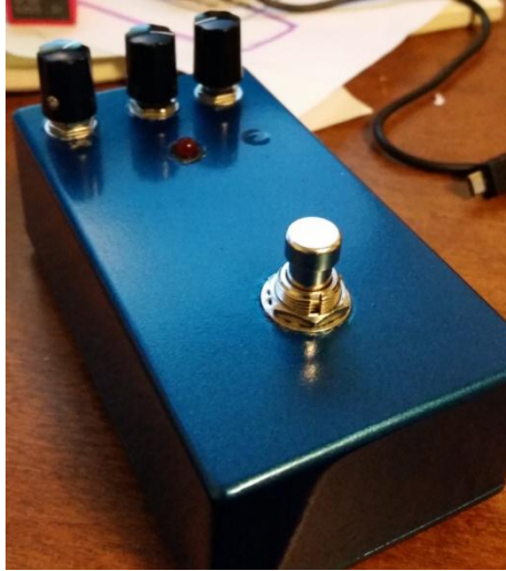
Figure 6.15: Enclosure with Paint Applied
