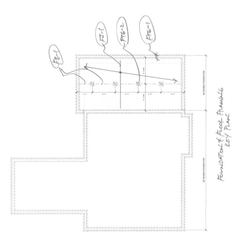
63.2 AT= 7'X (2)' = LOSE FLOOR FRAMING Kut = 20 SE 2 GOSE FJ-1 W=69.3PLF => NO REDUCTION ALCOURD W= (12PSF+40PSF) (16)=693PGF 1 7-0" 1 V= 42 - 69.3(7) = 24(3# M= al2 69.3 (72) = 425 1-# DEFLECTION A2 = 360 = 7K/2 = 0,23" Itoq = SwL4 384EAL = 5 (40 × 16)74 12 = 7.83) 12 4 384 EAL = 384 (1.64106)0.23 Controls Controcs Aptl = = 76/2 = 0.35" Itoo = 5WLY = 5(69.3)74/23 = 6.69 ind 384EABTL 384(1.64106)0.35 = 6.69 ind TRY 246 DE-L #2 I= 20,8 ml 5= 7.56 AL3 A = 8.25 m2
